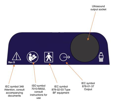
The output socket is for connection of the ultrasound transducer
