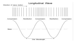
The diagram shows a sound wave travelling from left to right. The vertical bars represent thin slices of the medium which are displaced to form areas of compression and rarefaction. The sine wave represents their displacement relative to their mean position. The distance over which the vibration repeats itself is called the wavelength. The number of complete vibrations in one second is called the frequency of the sound wave.
