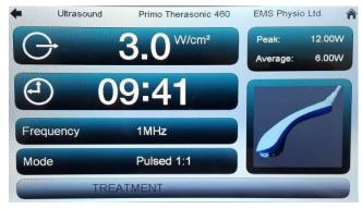
Move the transducer over the treatment site in small circular paths whilst setting the output intensity to the required level using the rotary control.
