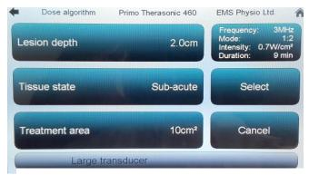
The data concerning the state of the area to be treated is chosen by stepping through the various button options. Once the relevant parameters have been entered touching Select will open a user screen loaded with the calculated treatment settings. Treatment is initiated by turning up the output intensity using the rotary dial, but it will be limited to the maximum Peak value previously calculated.
