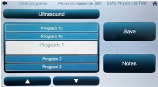
A screen will appear with a scrollable list of program slots – the active one is highlighted in the middle. Touching 'Save' will store the settings last open in the set up screen to this slot – if the slot isn't empty a pop-up window will appear asking you to confirm or cancel the save process (to prevent unintentional over-writing of a previously saved program).
