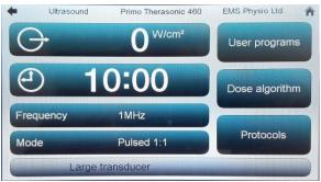
Touch the screen on the digits of the time display to increment some treatment time (maximum 30 minutes). Alternatively, touch the clock symbol to bring up the following screen:-
