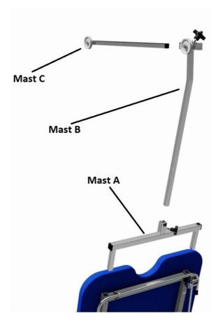
Mast A fits into the backrest of the couch. Elevate the backrest, check that there are no caps fitted which would prevent the mast fitting and slide the mast in. Ensure that the locking knob is facing you otherwise it will foul with the upholstery.
